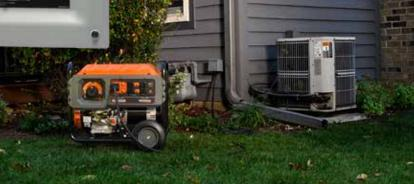
Plug one end of the cord into the 30 Amp outlet on the generator, and the other end into the power inlet box
